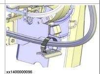
5 Fasten the cable package in the gripping clamps on the upper arm bracket.
