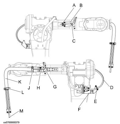
Α Rubber clamp with bracket В Bracket, right С Velcro strap D Upper arm cable package MH dressing Ε Rubber clamp with bracket F Connection plate G Bracket, left Н Rubber clamp with bracket J Gripping clamp (bracket left) Κ Protection hose L Gripping clamp (protection hose) М Air hose
